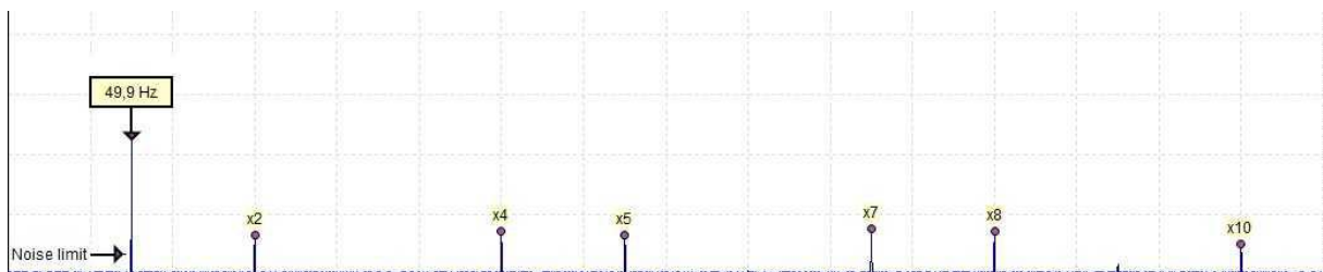
Family with harmonics. The 3 rd , 6 th and 9 th harmonics are missing, because there is not peak or the peak is lower then noise limit.
