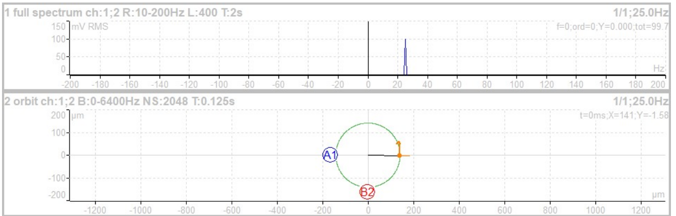
The vibration (orbit arrow) has the same direction as rotation.
